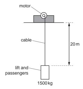
The lift and passengers have a combined mass of 1500 kg. The motor raises the lift through a distance of 20 m.
